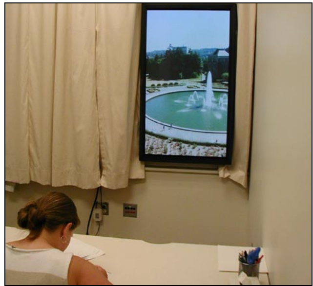
Figure 2. Person (demonstrator) working in an office with a “window of the future” – a large screen plasma display that is projecting real-time HDTV images of the local outdoor scene.
